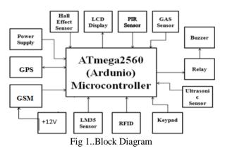
Fig.1. Shows the block diagram of the proposed method. In this Atmega2560 along with other peripherals Relay, LCD, PIR Sensor, GSM module, RFID module, IR Sensor, Level Sensor ,Phase detector ,Temperature Sensor & Humidity Sensor etc. Camera: The whole site room is under the cover of camera. It give inside images of BTS room & save it in PC. The site room includes door open/close sensor. IR Sensor for indicating the door open/close status.
