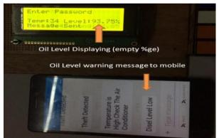
Fig 4 Low Diesel Level Indication SMS Sending to Technician Mobile respectively.
